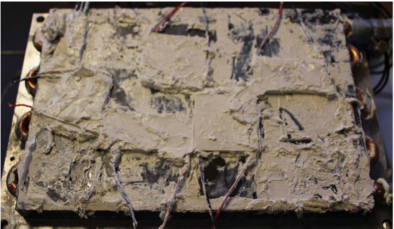
Figure 23. 5 TECs in paste on the liquid cooler (2014).
