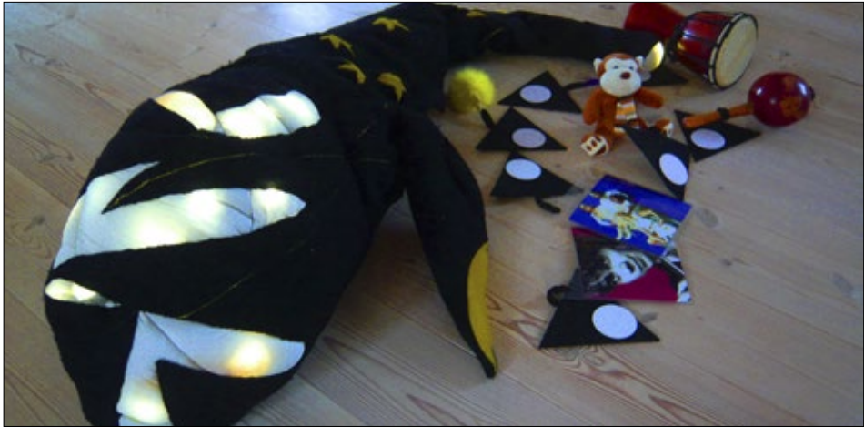
Picture 4: REFLECT's lumber-like soft things with RFID-tagged scene cards and tagged things to create choir sounds
