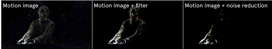
Figure 2: The motion image is improved by applying either a simple low-pass filter or a more advanced noise reduction filter.
