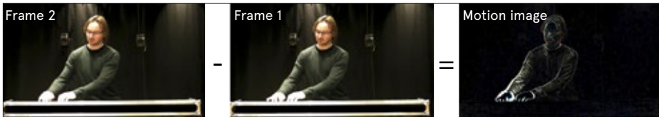
Figure 1: A motion image from a performance of a piano piece, recorded from the front: The motion image is created by subtracting subsequent frames in a video file (that is, looking at the difference between each individual pixel in two adjacent frames) looking at the difference between each individual pixel in two adjacent frames
